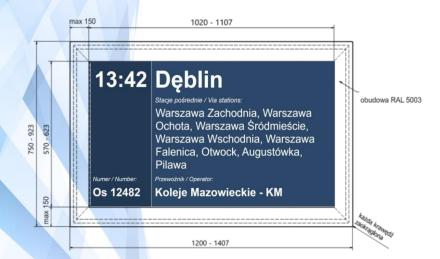
\* The content presented on the display and its arrangement is generated by CASDIP and is not the issue of the device supplier. For your reference, an example screenshot of the edge display is shown in the figure above
